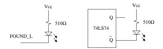
Figure 1 – LED Connections
